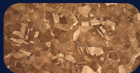
Wrought CNC structure etched 100x magnification
